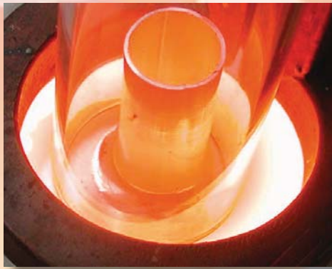
Induction Brazing of Stainless Steel in Protective Atmosphere (Brazing Temperature)
