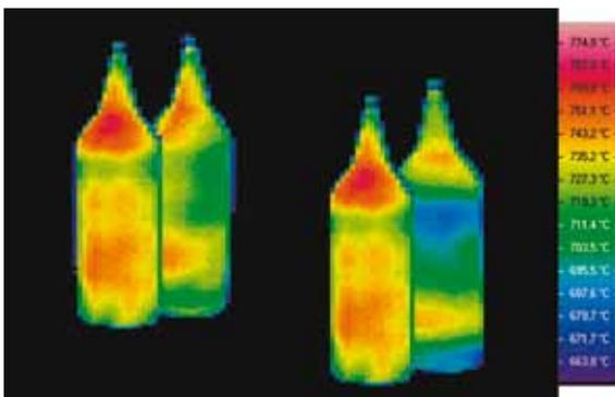
The shapes and temperature of glass are important measures to control process quality during glass container production.
