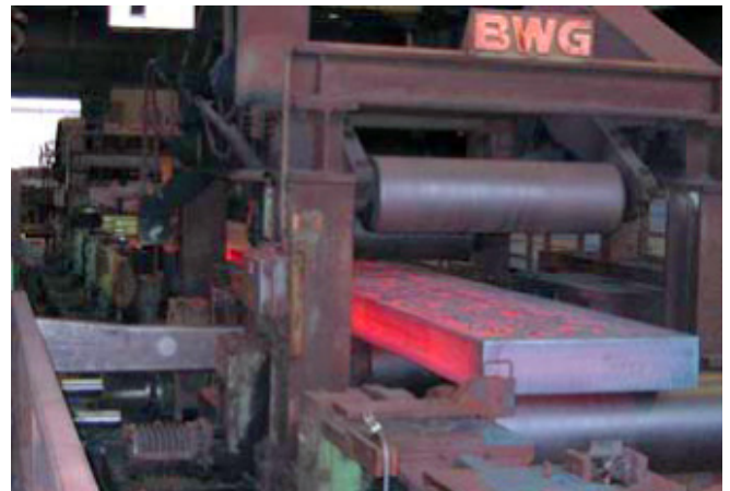
Figure 4: Automatic deburring machine
