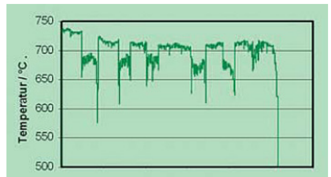
Figure 8: Temperature measurement of burr (measurement using a pyrometer)
