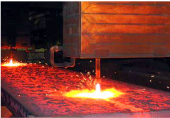
Figure 1: Lengthwise slab cutting
